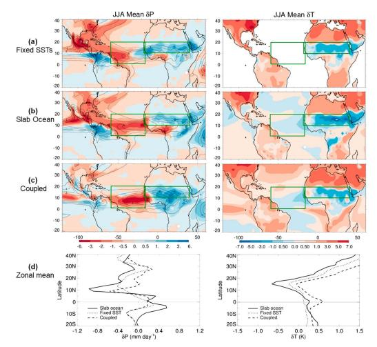
**Figure 2.** (left) JJA precipitation anomalies (10 ka-control, millimeter per day) in the three experiments: (a) fixed SSTs, (b) slab ocean, and (c) coupled dynamic ocean. (right) As above, but for temperature anomalies (K). In (d), anomalies are averaged over all longitudes. The green boxes delimit the North Atlantic Intertropical Convergence Zone and Sahel regions. The color bar intervals are pseudo-logarithmic. JJA = June, July, August; SST = sea surface temperature.
