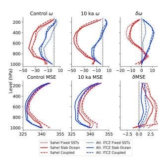
**Figure 3.** June, July, August vertical profiles of (top row)  $\omega$  (hPa/day) and (bottom row) MSE (K) in the control and 10 ka simulations, and their anomalies (10 ka-control). Results are averaged over the Sahel and North Atlantic ITCZ regions. MSE = moist static energy; SST = sea surface temperature; ITCZ = Intertropical Convergence Zone.
